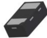
DFN1006-2L (Bottom View)
